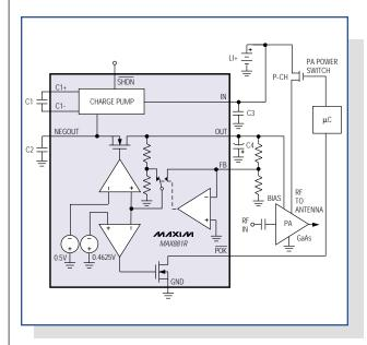
Figure 3. An interlock feature of the MAX881R protects the GaAs PA from damage.
