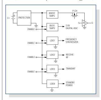
Figure 1. Switch-mode and linear regulators distribute power cleanly and efficiently.
