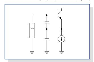
Figure 1. The basic Colpitts oscillator
