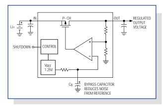
Figure 4. Output noise from an LDO regulator is reduced by adding a bypass capacitor (C<sub>B</sub>) to the voltage reference.
