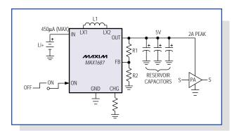
Figure 2. For burst systems such as IS-136 and GSM, large transients on the battery are minimized by reservoir capacitors and a boost converter.
