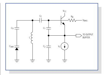
Figure 2. Use of the Colpitts topology in a VCO
