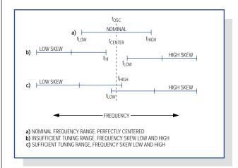
Figure 5. Tuning range and frequency shifts
